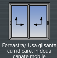
Fereastră/ Usa glisanta in doua canate mobile (imbinarea cercevelor la 90 grade)
