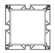
/ 250x250mm mullion, i.e., steel or concrete body surrounded with aluminium profiles. (01)
