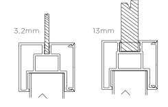
/ Special profiles with two different inserting channels on both sides, i.e. 3/25mm and 13/25mm, which allow combination of decorative surfaces (glass, wood, metal) at any point of the panel. (03)
