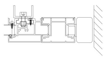
/ The opening mechanism is attached on a special transom profile to add extra strength against loosening and damaging problems after a long period of time.
