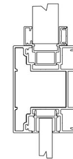
/ Glazing installation with the use of special profile which shortens the gap from 25mm to 13mm.
