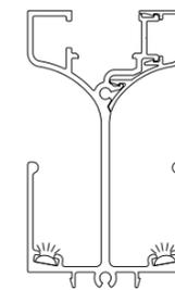
/ Integrated handle in the door leaf, with the option of concealed lighting at both sides.
