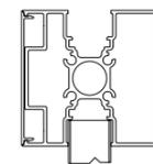
/ 80x80mm mullion, simple or corner, combined with caps or handrail, with special design and concealed fixing points. (03)
