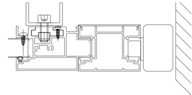
/ The opening mechanism is attached on a special transom profile to add extra strength against loosening and damaging problems after a long period of time.
