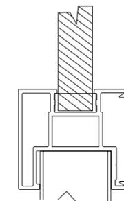
/ Special profile for "random" glazing placement between the aluminium louvers.
