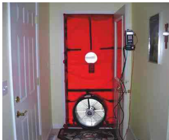
Figure 5.4 Blower door test
